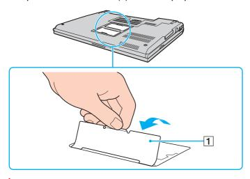
The insulation sheet is equipped for module protection. Do not pull it too hard to damage the sheet.
